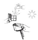
Grasp recessed area on each side of the dry filter and pull upward. Rinse under running water and must be completely dry before recombining with the lid of the DWT.
