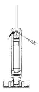
In the event that the product must be returned, please disassemble the handle. Press the spring to release the handle with a tool (like a screwdriver) and lift the released handle from the appliance.
