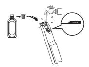
Open the tank cap, and fill with tap water to the Max line. When deep cleaning is necessary, add one bottle cap of solution to the CWT and tightly close the cap.
