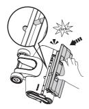
When replacing, always latch the brush cover into place to avoid leakage.
